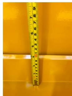
Some 'fixed sumps' are not sealed to the cabinet walls, which leaves a risk of a spill running down the back of the cabinet, missing the sump and leaking out through the base of the cabinet.
