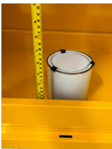
Some sumps are quite shallow at just 80mm. This provides a lower capacity sump, which is more easily breached.
