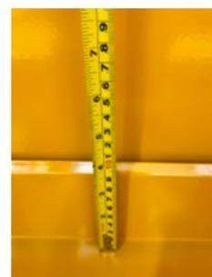
Some 'fixed sumps' are not sealed to the cabinet walls, which leaves a risk of a spill running down the back of the cabinet, missing the sump and leaking out through the base of the cabinet.
