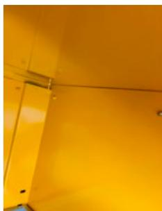
With some riveted cabinets you can see daylight through the corners.
