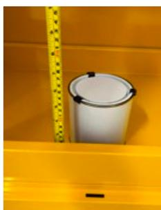
Some sumps are quite shallow at just 80mm. This provides a lower capacity sump, which is more easily breached.
