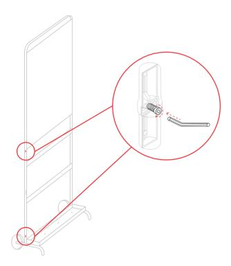
Once all parts are in position, tighten all expanders (A+B) with an allen key to secure the complete frame.
