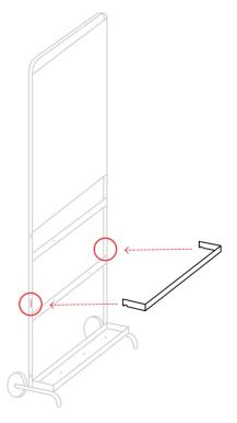
6. Optional – hook the fire extinguisher protector frame into either side of **Part 1.**
